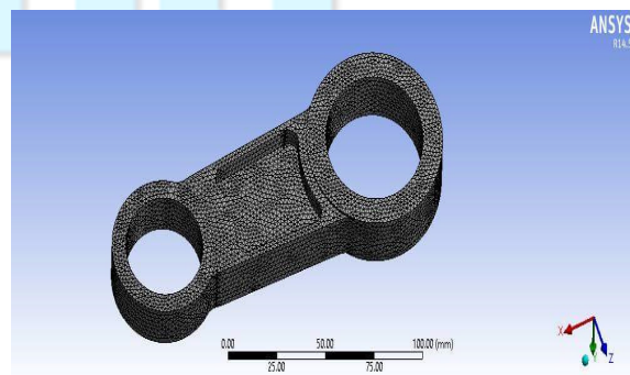
Fig 7: Mesh model of connecting rod
